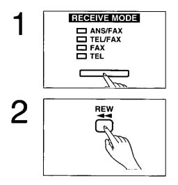
Press the **RECEIVE MODE** button until the ANS/FAX indicator lights.
