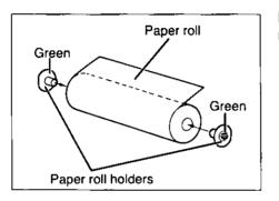
Fix the paper roll holders on both sides of the recording paper roll.
