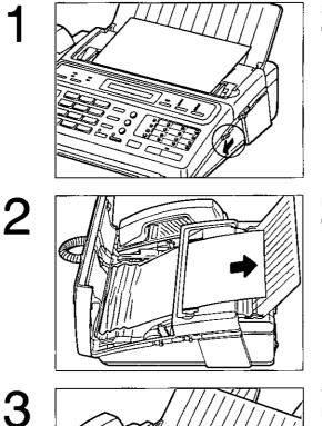
Slide the **FRONT LID OPEN** lever forward to open the document feeder unit.
