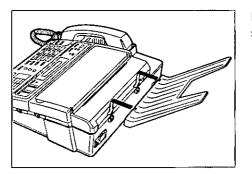
Insert two fins of the tray into holders on the rear side of the unit.
