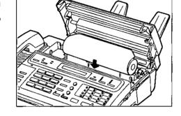
Place a recording paper roll into the paper compartment.
