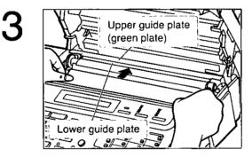
Insert the leading edge of recording paper between the upper guide plate (green plate) and the lower guide plate.
