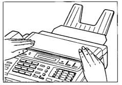
Then insert its leading edge between upper and lower guide plate and pull the paper a few centimeters (one or two inches) out of the unit.
