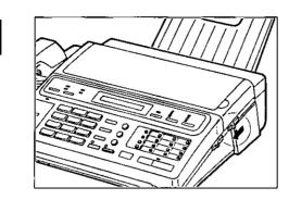
Slide the **BACK LID OPEN** lever forward to open the paper compartment cover.
