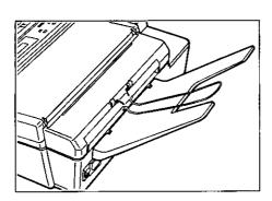
Insert two hooks of the diverter into holders on the rear side of the unit.
